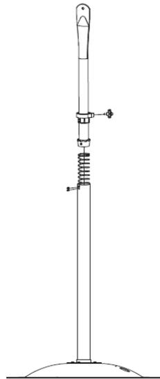
2. Insert the spring into the lower pole as shown in the picture and assemble the upper pole.
