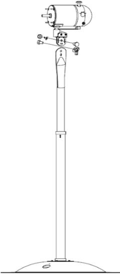
3. Assemble the motor.
