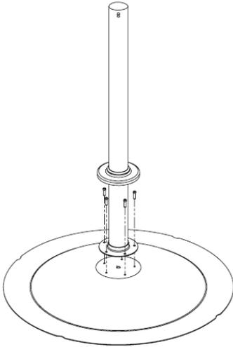
1. Attach the lower pole to the base and tighten it by using the screws on the base
